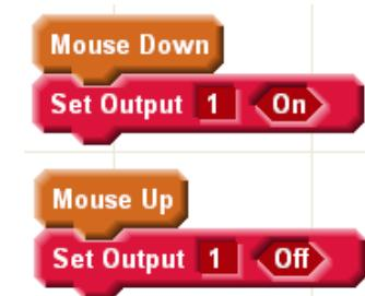
**Step 17)** Click the button and wait for the status to indicate "Running". Click and hold the "Test Button" down. Your load should be active. Release the mouse and the load should be inactive.
