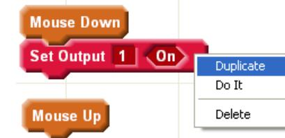
**Step 16)** Place the duplicated block under the "Mouse Up" Block. Click on the "On" diamond field and choose "Off".
